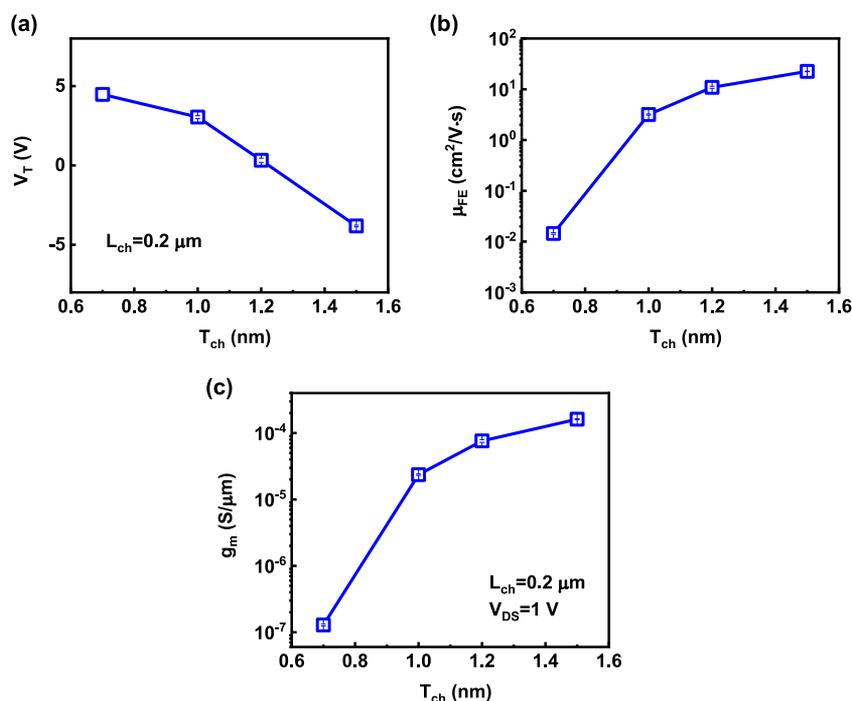
**Figure 3.** (a) Threshold voltage, (b) field effective mobility, and (c) transconductance at  $V_{DS} = 1 \text{ V}$  versus channel thickness of  $\text{In}_2\text{O}_3$  MOSFETs with channel length of  $0.2 \mu\text{m}$ . Each data point represents the average of at least 5 devices.
