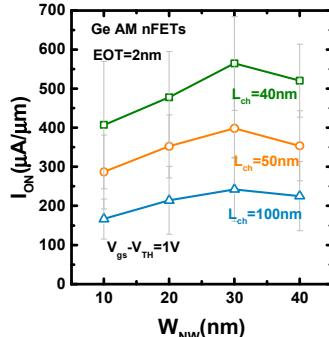
**Fig. 17**  $W_{NW}$  dependence of the  $I_{ON}$  of AM Ge nanowire nFETs with an EOT of 2 nm. The  $I_{ON}$  first increases and then decreases with reduced  $W_{NW}$ .
