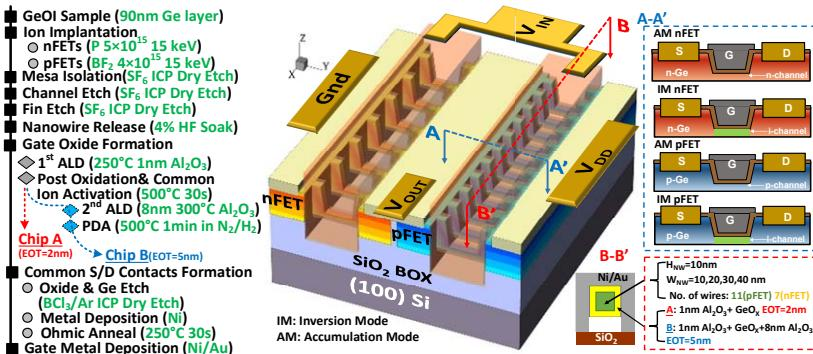
**Fig. 1** Fabrication process flow of the Ge nanowire CMOS. Splits on gate oxide are studied.
