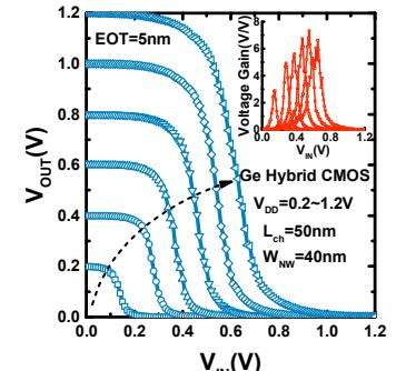
**Fig. 27**  $V_{OUT}$  versus  $V_{IN}$  of the same CMOS inverter shown in Fig. 25. The inset shows the voltage gain.
