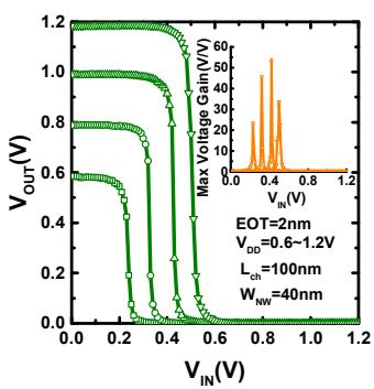
**Fig. 28**  $V_{OUT}$  versus  $V_{IN}$  of a 100 nm  $L_{ch}$ , 40 nm  $W_{NW}$  and 2 nm EOT Ge nanowire CMOS inverter with highest voltage gain of 54 V/V given in inset.
