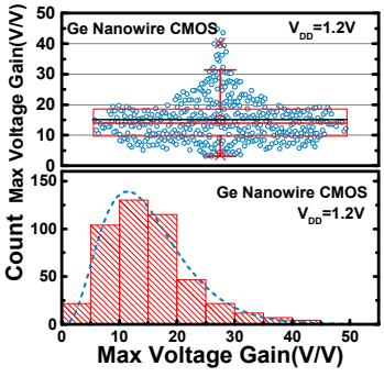
**Fig. 31** BOX plot and histogram for the maximum voltage gain of Ge nanowire CMOS inverter at  $V_{DD}$  of 1.2 V, based on more than 400 measured devices.
