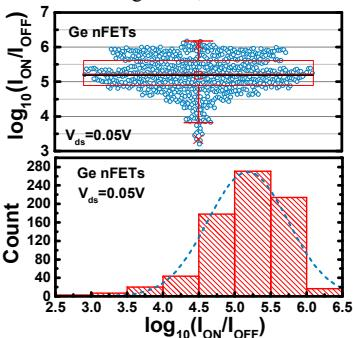
**Fig. 12** BOX plot and histogram for the  $\log_{10}(I_{ON}/I_{OFF})$  of Ge nanowire nFETs at  $V_{ds}$  of 0.05 V. based on more than 800 measured data points.
