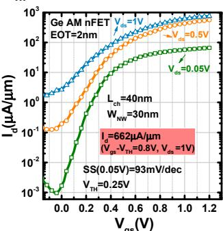
**Fig. 13** Transfer curves of a 40 nm  $L_{ch}$  and 30 nm  $W_{NW}$  Ge AM nanowire nFETs with  $I_{ON}$  of 662  $\mu\text{A}/\mu\text{m}$  at  $V_{ds}$  of 1 V and  $V_{th} = 0.8$  V.
