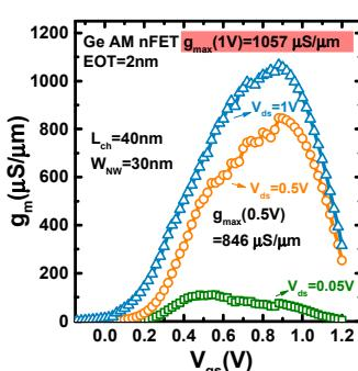
**Fig. 14**  $g_m$  vs.  $V_{gs}$  curves of the same Ge AM nanowire nFETs given in Fig. 13 with 40 nm  $L_{ch}$  and 30 nm  $W_{NW}$ . Record high  $g_{max}$  of 1057  $\mu\text{S}/\mu\text{m}$  is obtained.
