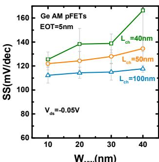
**Fig. 24**  $W_{NW}$  dependence of the SS of AM Ge nanowire pFETs with EOT of 5 nm. Smaller  $W_{NW}$  devices have better SS.
