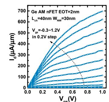
**Fig. 15** Output curves of the same Ge AM nanowire nFETs given in Fig. 13 with 40 nm  $L_{ch}$  and 30 nm  $W_{NW}$ . The  $I_{max}$  is around 700  $\mu\text{A}/\mu\text{m}$ .
