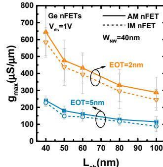
**Fig. 18**  $g_{max}$  scaling metrics of AM and IM Ge nanowire nFETs with an EOT of 2 and 5 nm. The  $g_{max}$  first increases and then decreases with reduced  $L_{ch}$ .
