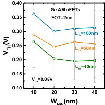
**Fig. 9**  $W_{NW}$  dependence of the  $V_{th}$  of AM Ge nanowire nFETs with an EOT of 2 nm. Smaller  $W_{NW}$  devices have larger  $V_{th}$ .
