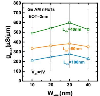
**Fig. 19**  $W_{NW}$  dependence of the  $g_{max}$  of AM Ge nanowire nFETs with an EOT of 2 nm. The  $g_{max}$  first increases and then decreases with reduced  $W_{NW}$ .
