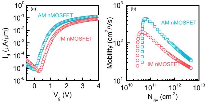
**Fig. 2.** (a)  $I_d$ - $V_g$  curves of AM and IM Ge nMOSFETs with  $10 \mu\text{m}$   $L_{ch}$  and  $100 \mu\text{m}$   $W_{ch}$  at  $V_d$  of  $0.05$  V; (b) Electron mobility versus  $N_{inv}$  curves of AM and IM Ge nMOSFETs. AM MOSFET shows better ON-state current and higher electron mobility.
