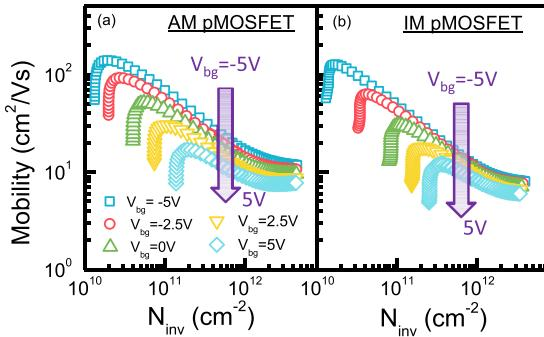
Fig. 5. Hole mobility vs.  $N_{\text{inv}}$  in (a) AM and (b) IM pMOSFETs under various  $V_{\text{bg}}$  (from  $-5 \text{ V}$  to  $5 \text{ V}$ ). Hole mobility decreases under positive  $V_{\text{bg}}$ .
