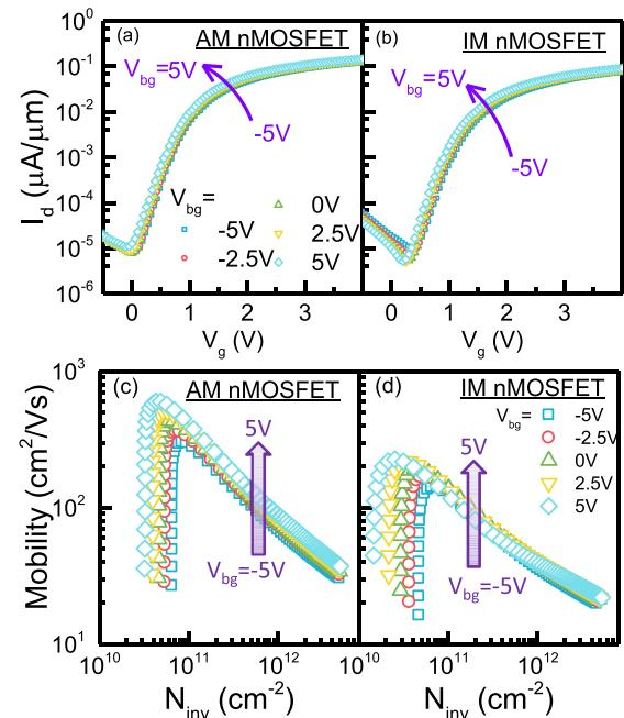
**Fig. 4.**  $I_d$ - $V_g$  curves of (a) AM and (b) IM nMOSFETs under various  $V_{bg}$  (from  $-5$  V to  $5$  V) at  $V_d$  of  $0.05$  V; Electron mobility vs.  $N_{inv}$  in (c) AM and (d) IM nMOSFET under various  $V_{bg}$  (from  $-5$  V to  $5$  V).  $I_d$  and electron mobility increase under positive  $V_{bg}$ .
