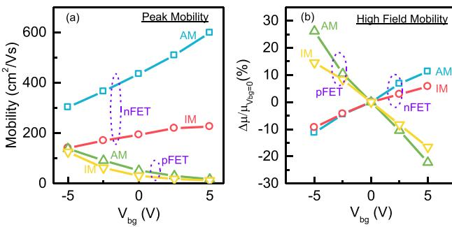
Fig. 6. (a) Peak carrier mobility and (b) the change of high field carrier mobility ( $N_{\text{inv}} = 5 \times 10^{12} \text{ cm}^{-2}$  for electron,  $N_{\text{inv}} = 2 \times 10^{12} \text{ cm}^{-2}$  for hole) in AM nMOSFET, IM nMOSFET, AM pMOSFET and IM pMOSFET under  $V_{\text{bg}}$  from  $-5 \text{ V}$  to  $5 \text{ V}$ .
