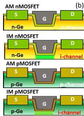
**Fig. 1.** (a) Key fabrication process of the GeOI MOSFETs with recessed channel and source/drain; (b) Cross section views of devices with four types of operation mode: AM nMOSFET with n-channel, IM nMOSFET with i-channel, AM pMOSFET with p-channel and IM pMOSFET with i-channel.
