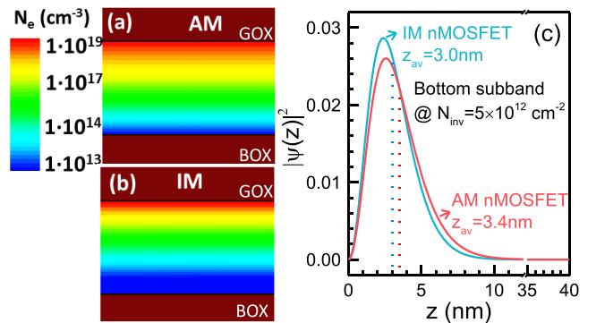
**Fig. 3.** Simulated on-state ( $V_g - V_{th} = 1$  V) electron distribution inside the channel in (a) AM and (b) IM nMOSFET; (c) self-consistent result of  $|\Psi(z)|^2$  versus  $z$  in AM and IM nMOSFETs with  $N_{inv}$  of  $5 \times 10^{12} \text{ cm}^{-2}$ . AM nMOSFET has higher electron concentration and larger  $z_{av}$ .
