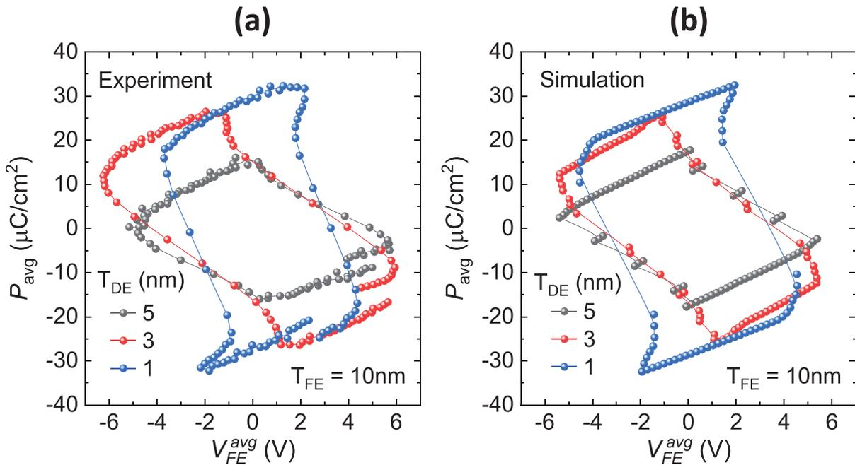
**FIG. 4.** Extracted average polarization ( $P_{avg}$ ) vs average voltage across the FE layer ( $V_{FE}^{avg}$ ) in the FE-DE stack from the (a) experimental and (b) simulated  $P_{avg}$ - $V_{app}$  characteristics.
