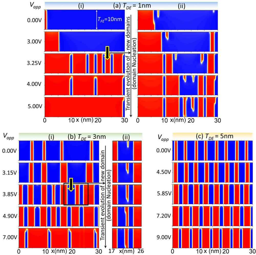
**FIG. 3.** Simulated polarization profile in FE at different applied voltages ( $V_{app}$ ) in FE-DE stacks for different  $T_{DE}$  = (a) 1 nm, (b) 3 nm, and (c) 5 nm showing domain nucleation and domain-wall motion-based polarization switching. In all the cases, the FE thickness is 10 nm.
