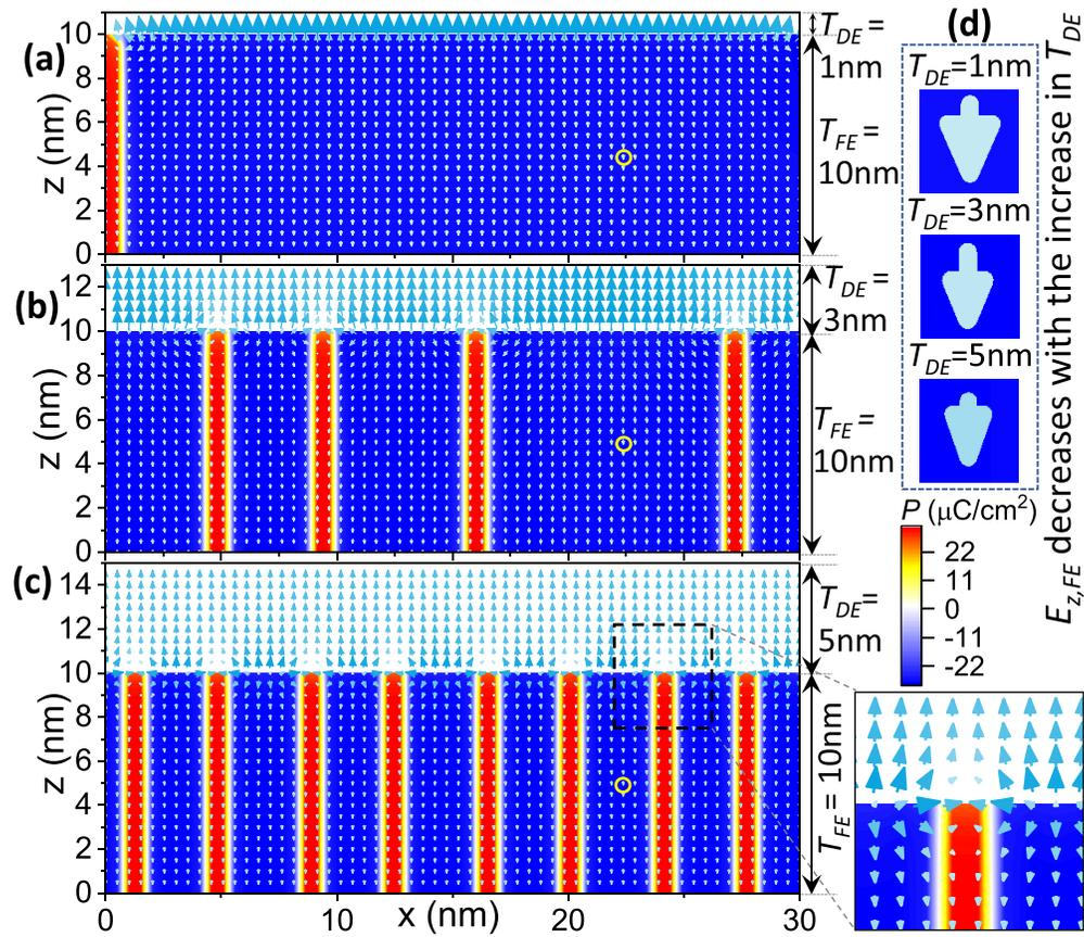
**FIG. 2.** Simulated  $P$  (color map) and  $E$ -field (arrow) profile in FE-DE stacks for  $T_{DE} =$  (a) 1 nm, (b) 3 nm, and (c) 5 nm. The blue (red) regions signifying  $-P$  ( $+P$ ) domains. (d)  $E_{z,FE}$  at the yellow circled points shown in (a)–(c) signifying the decrease in the depolarization field within the FE with the increase in DE due to the formation of a larger number of reverse domains.
